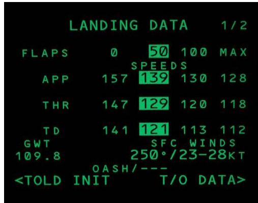
Figure 3. Recreation photo of CNIMU displaying 50% flap approach speeds
