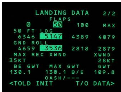
Figure 4. Recreation photo of CNIMU displaying 50% flap landing distance
